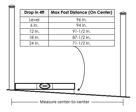
Determine the amount of vertical drop in a 4' horizontal distance by placing a 48" level on the ground, raising it until it is level, and then measuring from the bottom of the level to the ground. Consult the chart to the left for the maximum post spacing (center-to-center).
