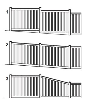
1 STEP METHOD: This fence gradually "steps" down the slope so each section is the same length and the rails remain level. Gaps will exist under the fence. The downhill post will need to be set higher to allow attachment of the top rail. Taller posts may be required. When laying out the fence spacing between posts, the distance must be measured horizontally and not parallel to the ground.
