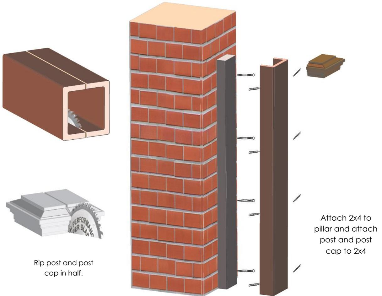
1. Using a table saw, rip one side of the post in half. Flip the post over to rip the other side. Keep the same edge against the guide to insure an even cut.
