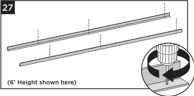
27. Remove each L-channel, and predrill holes at the locations marked in step 26 using a 1/8" drill bit. **DO NOT** predrill the posts.
