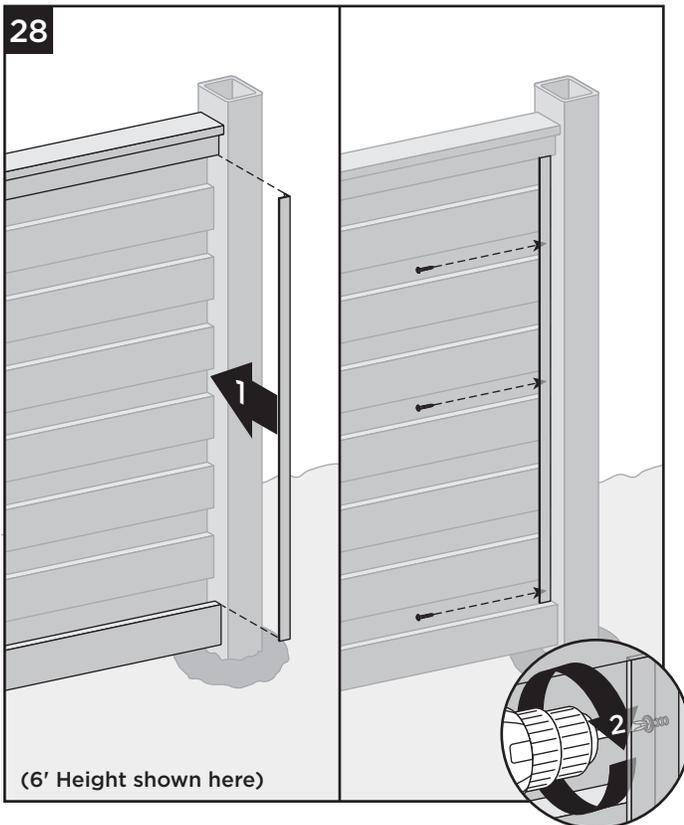
28. Replace each L-channel in same location as in steps 25/26, and attach to the post using (1) #8 x 1" pan head screw at each predrilled location.
