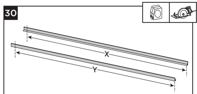
30. Cut the remaining (2) aluminum L-channels individually to the lengths measured in the previous step.
