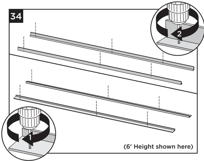
34. Remove each L-channel, and predrill holes at the locations marked in steps 32 and 33 using a 1/8" drill bit. **DO NOT** predrill posts or pickets.
