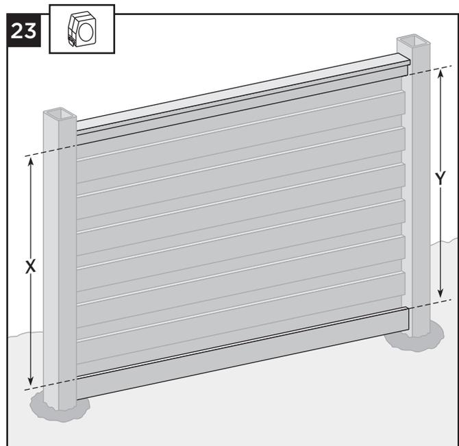
23. Measure the distance between the top and bottom rails on the **FRONT** side of the fence assembly.
