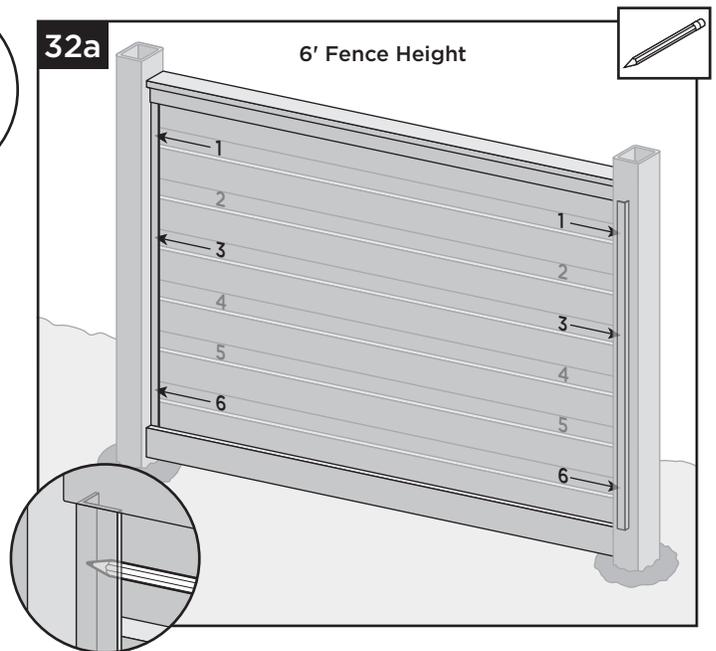
**32a.** Marking L-channels for attachment to posts on BACK side for 6' fence height: Mark (3) locations on each L-channel, starting from the top, mark the 1st, 3rd and 6th openings in the infill where the L-channel's short leg is visible.
