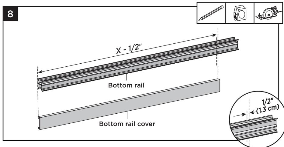
8. Cut the aluminum bottom rail 1/2" shorter than the bottom rail covers.
