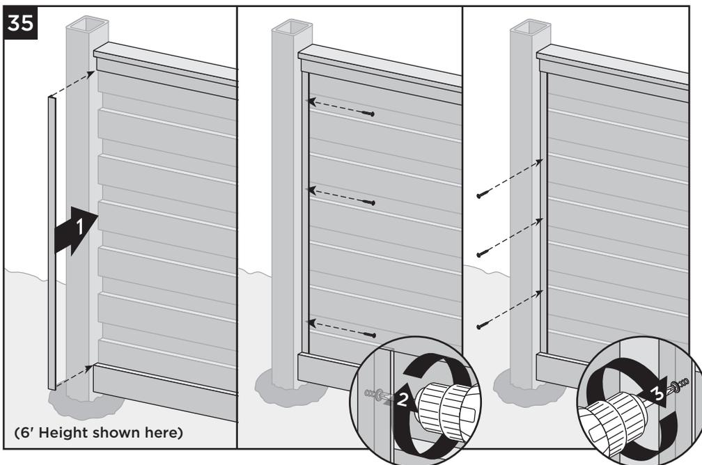
35. Replace each L-channel in same location as in steps 31/32, and attach to the post and pickets using (1) #8 x 1" pan head screw at each predrilled location.
