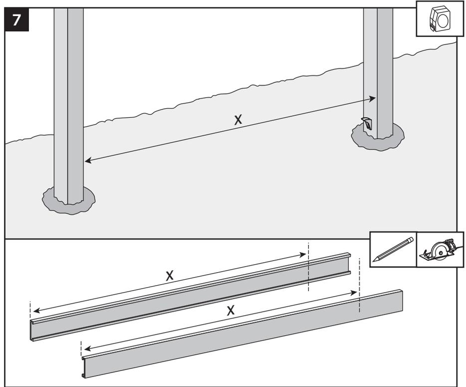
7. Measure the distance between the posts, and cut the bottom rail covers to length.
