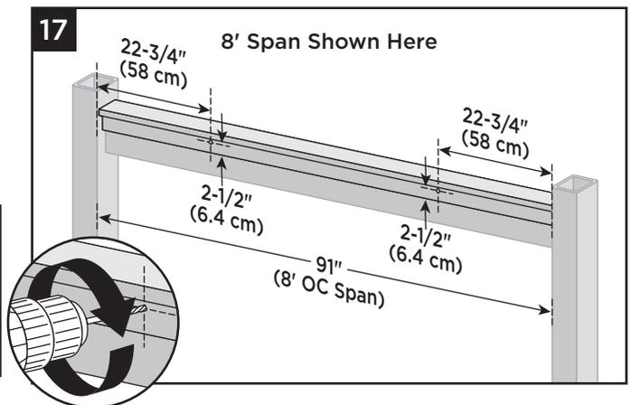
17. On the **BACK** of the fence assembly, predrill thru the aluminum insert using a  $\frac{1}{8}$ " drill bit at the quarter points of the top rail approximately  $2\frac{1}{2}$ " from the bottom edge of the rail. Adjust quarterpoint measurements accordingly for smaller post spans.
