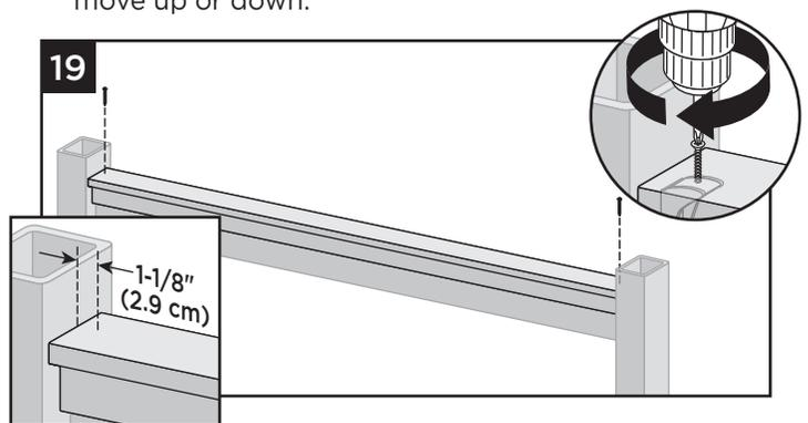
19. Measure approximately  $1\frac{1}{8}$ " out from each post and attach the top rail to the top brackets using (1) #8 x  $1\frac{5}{8}$ " flat head screw per bracket.
