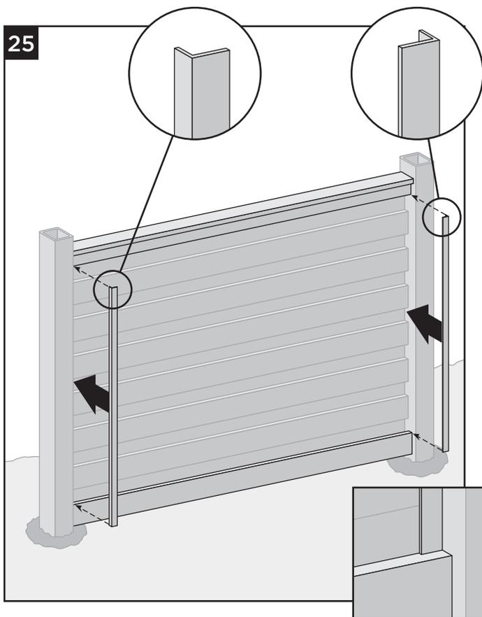
**25.** Position each L-channel against the post with the short leg against the post and the long leg extending over the pickets. Insert the short leg between the post and the ends of the pickets so the long leg is flush against the pickets and aligned with the inside edge of the top and bottom rails.
