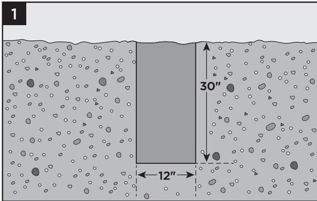
1. Dig holes for posts 12" in diameter and 30" deep **MINIMUM** (or as required per local codes or conditions). Holes should be dug to allow for equal amount of concrete on all sides of the posts.
