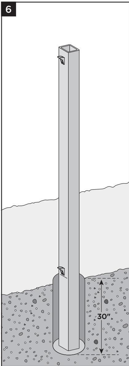
6. Set the posts at the desired spacing with an embedment of 30". Ensure posts are plumb and level. Fill holes with code approved concrete and allow this to fully set before attaching fence components.
