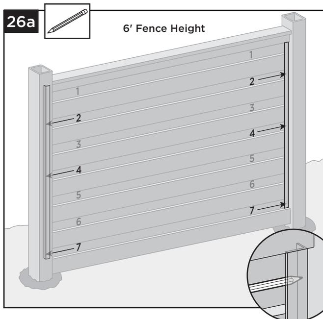
**26a.** Marking L-channels for attachment to posts on FRONT side for 6' fence height: Mark (3) locations on each L-channel, starting from the top, mark the 2nd, 4th and 7th openings in the infill where the L-channel's short leg is visible.
