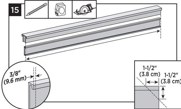
15. Cut the first picket  $\frac{3}{8}$ " shorter than the top rail. In addition, notch both ends of the first picket at  $1\frac{1}{2}$ " x  $1\frac{1}{2}$ " x  $45^\circ$ .
