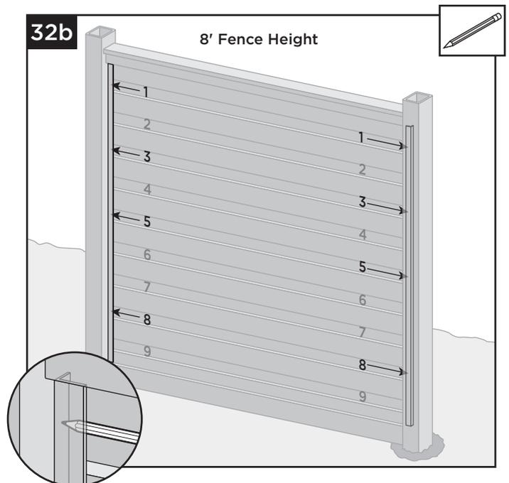
**32b.** Marking L-channels for attachment to posts on BACK side for 8' fence height: Mark (4) locations on each L-channel, starting from the top, mark the 1st, 3rd, 5th and 8th openings in the infill where the L-channel's short leg is visible.
