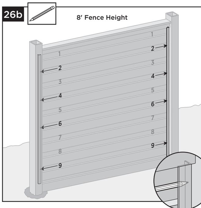
**26b.** Marking L-channels for attachment to posts on FRONT side for 8' fence height: Mark (4) locations on each L-channel, starting from the top, in the 2nd, 4th, 6th and 9th openings in the infill where the L-channel's short leg is visible.
